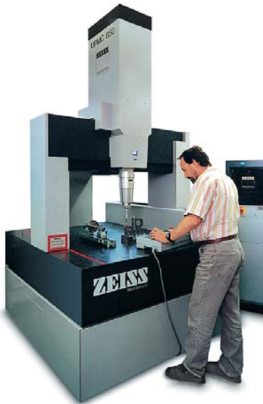
precision on the workpiece: 5 \mu m, unmanned production
