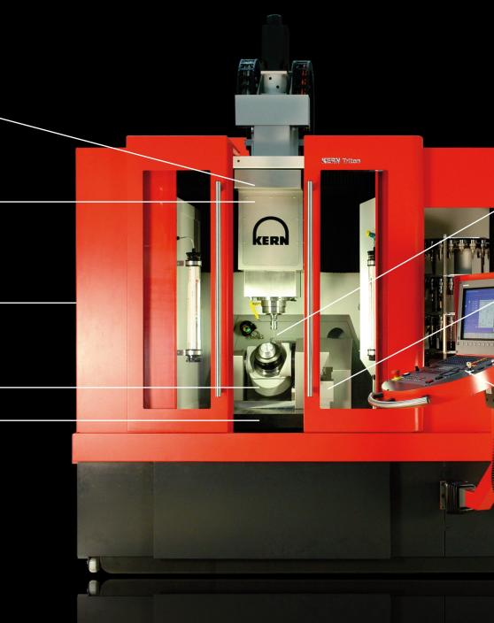
Eliminate thermal effects: A central temperature management system ensures temperature control of the spindle, axes, metalworking fluid, hydraulics, machine base and electrical cabinet with a regulation accuracy of < ±0.25 K
